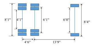
**Figure 4: Load Test Truck Dimensions**
