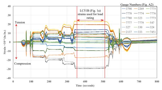
Figure 5: Strains for load case LC51B
