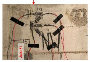
(b) Gauges mounted on wall
