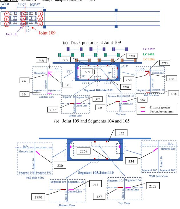
Joint 109: Flexure RF = 0.66, Principle Stress RF = 1.24
